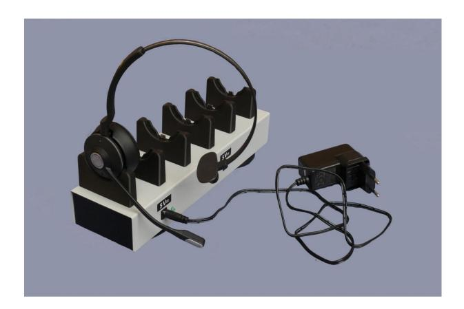
Then insert the power adapter into a 240 V AC, 50.60 Hz socket. The supply voltage is indicated by a green LED diode, which is located next to the 5V =socket on the rear panel. When the green LED is on, then the charger is ready to use.
